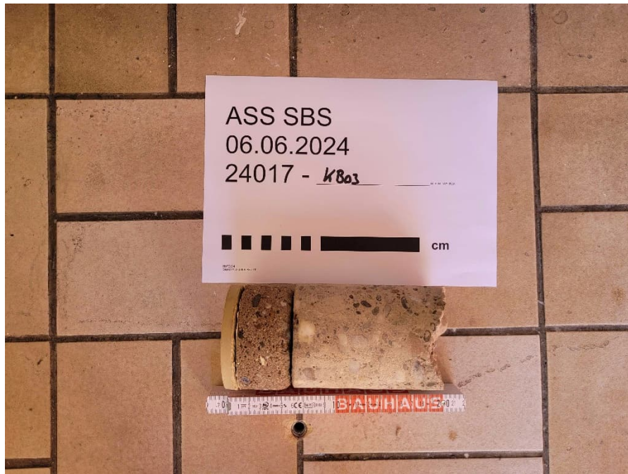
EG, WC-Vorraum, Kernbohrung 03 12mm Fliesenbelag, 45mm Estrich, >140mm Beton
